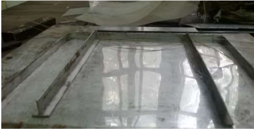
Figure 3. 4: Arrangement of aluminium frame and die
