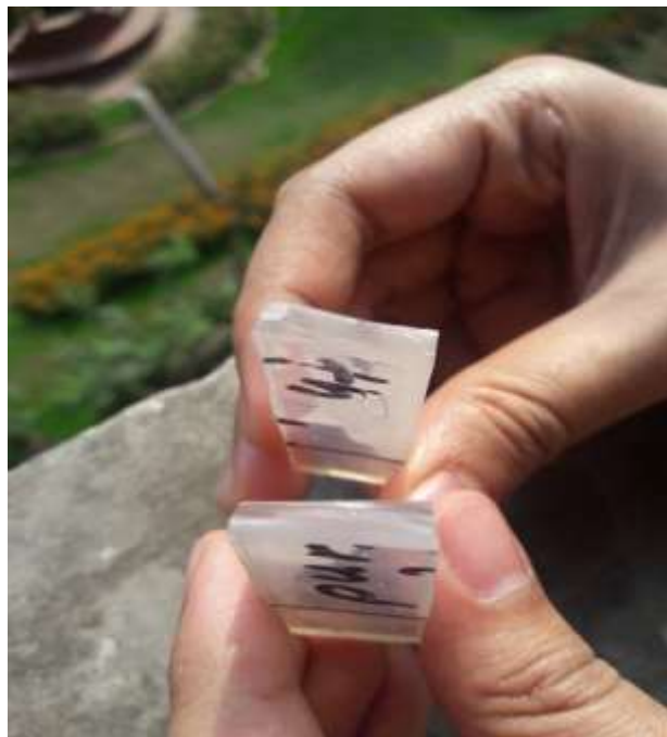
Figure4. 34: Fracture surface of pure polyester casting
