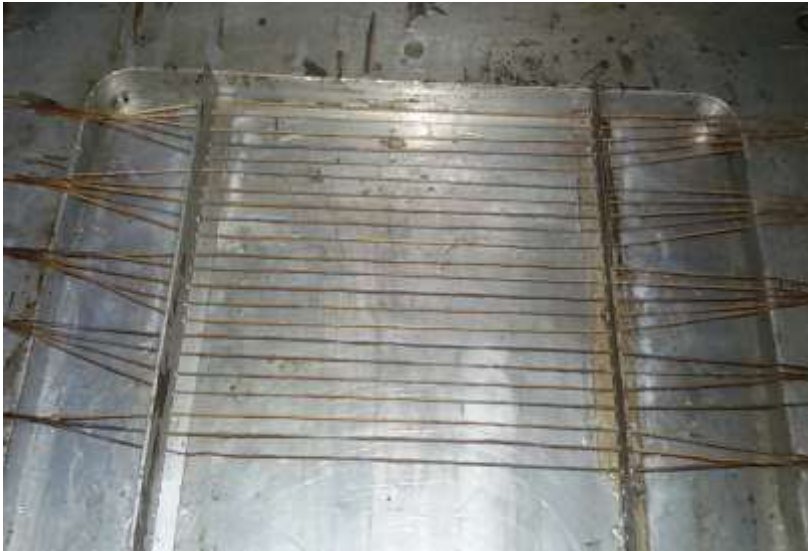
Figure 3. 6: Completion of fiber Arrangement
