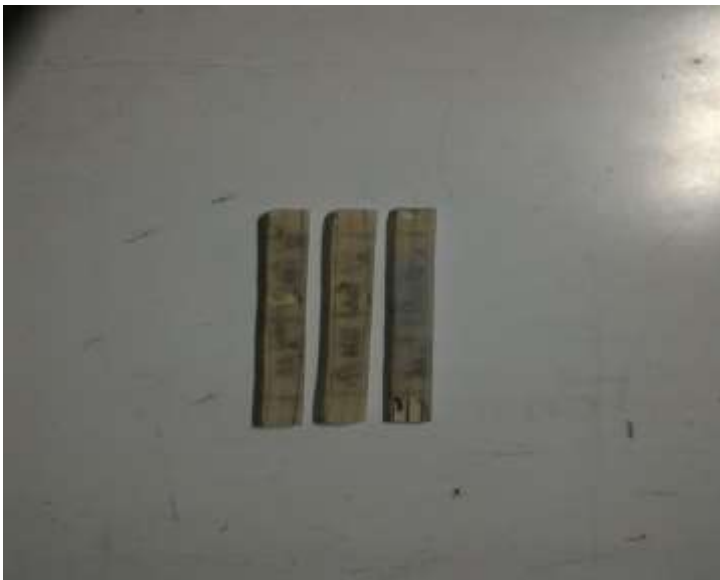
Figure 3. 13: Specimen for flexure test
