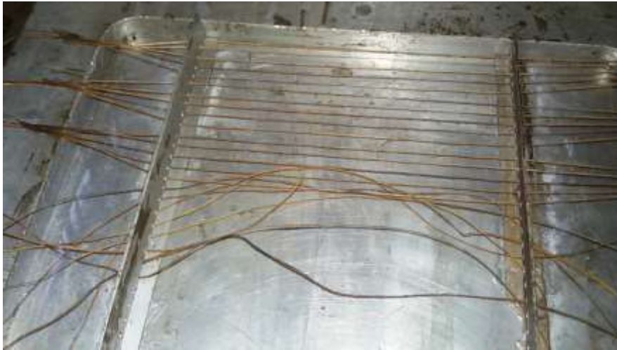
Figure 3. 8: Various stages of fiber alignment
