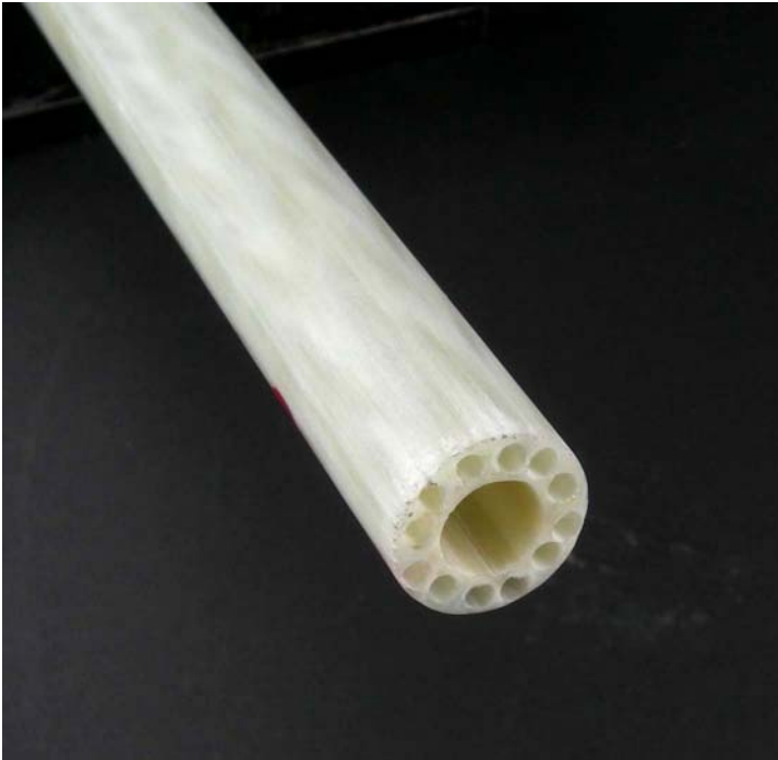
9.24 Braid-pultruded 'technical plant stem.'
