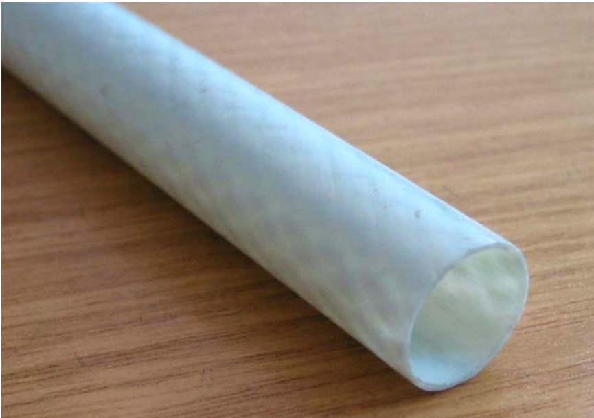
9.21 Braid-pultruded tubular profile with thermoset matrix.
