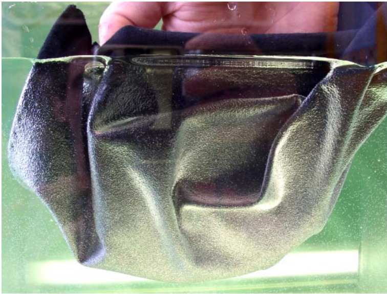
10.3 Textile made of bulky special yarn with especially good air-storing property.
