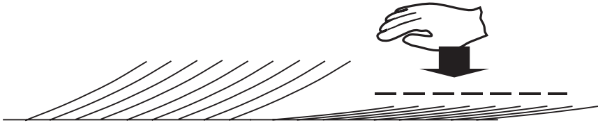
(a) Shape of fine fibres under compression
