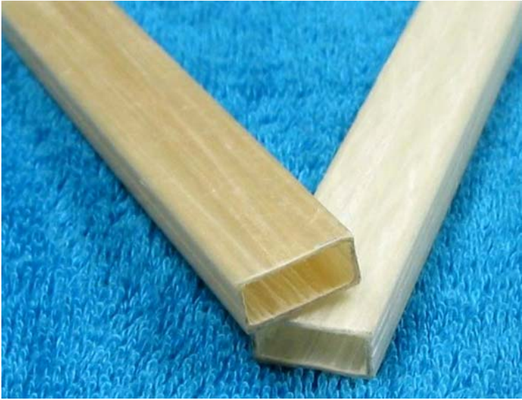
9.20 Thin-walled, unidirectional, reinforced thermoplastic profile produced by pultrusion.
