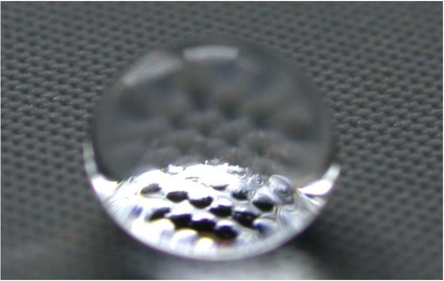
7.3 Water drop on superhydrophobic textile surface.
