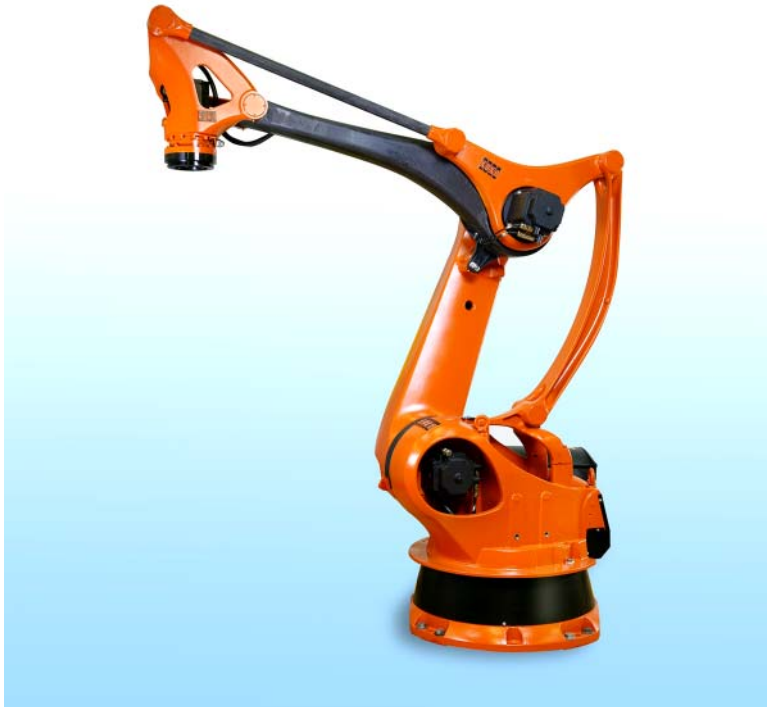
9.4 Extremely lightweight carbon fiber/reinforced plastics robot-arm, produced by tailored fiber placement (courtesy of Kuka GmbH, Germany).
