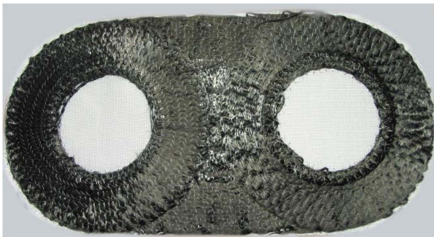
9.5 Example of a tailored fiber placement preform.
