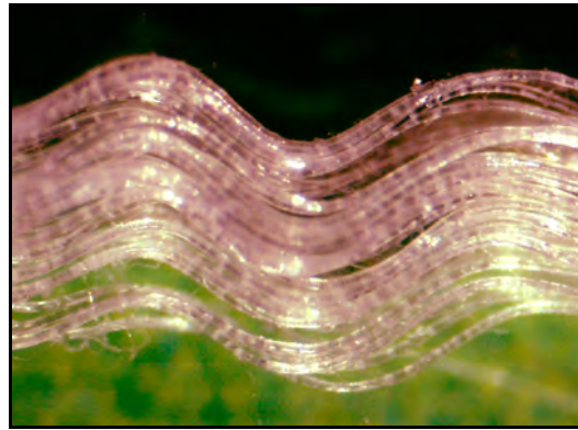
Figure 18. Enlarged View of a Continuous Multifilament, Crimped Yarn Extracted from a Plain-Woven Fabric
