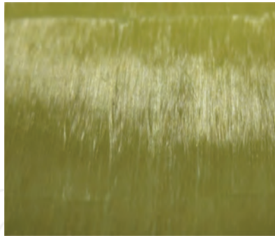
Figure 7. Ballistic panel Gold Shield® GV-2018 with Kevlar® by Honeywell; source: author's own photo archives. Note: The sample is composed of two panels and each of the panels consists of two layers. The first layer consists of sets of the parallel yarns positioned vertically (V) and the second layer contains the yarns positioned horizontally (H). Thus, the scheme of the sample construction is: (V + H) + (V + H). Total area density: 510 g/m 2 . Thickness: 0.78 mm.
