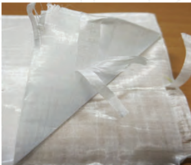
Figure 12. Ballistic panel Spectra Shield® SR-1226 by Honeywell. The sample is delaminated/stratified, showing two panels with two layers each, and the yarns in each panel are positioned perpendicularly; source: author's own photo archives.
