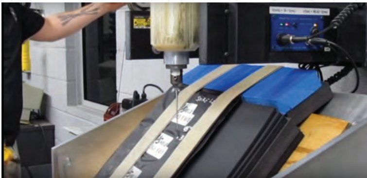
Figure 26. Stab-Resistant Panel NIJ 0115.00 Level II Spikes Test; source: http://www.aashield.com/ .
