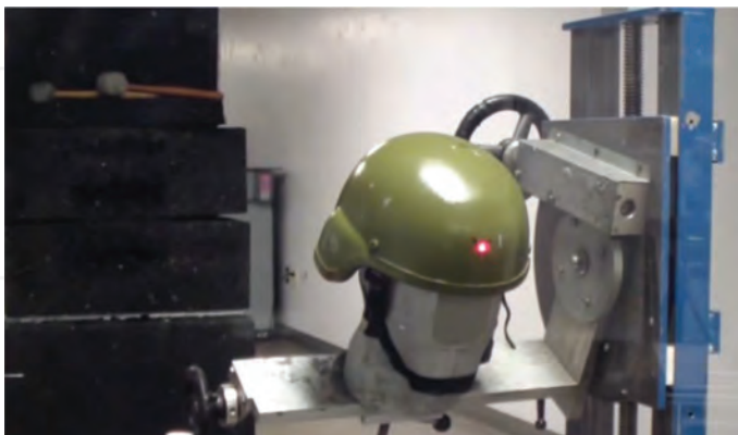
Figure 25. A ballistic test set up for testing a MICH ballistic helmet against 9 mm calibre; source: www.kick-az.com .
