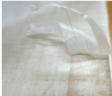
Figure 14. Spectra Shield® II SA-4144 panel by Honeywell. The sample is delaminated/stratified, showing two separate panels with two layers of yarns in each of them, positioned perpendicularly; source: author's own photo archives.
